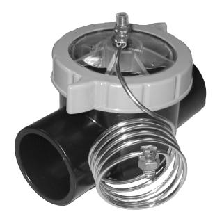
The zinc anode will gradually sacrifice itself over time. When it has depleted itself it may be replaced by removing the top cover and replacing the anode. No re-plumbing is required. Replacement anode is CMP 25810-200-950.
