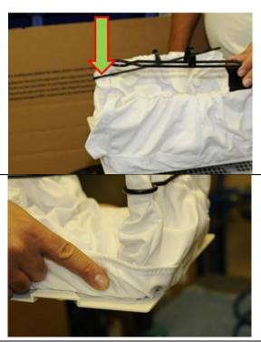
6. When putting filter bag back in place, ensure that the elastic band is completely down over the lip at the base of the bottom plate to prevent dirt and debris from escaping bag.
