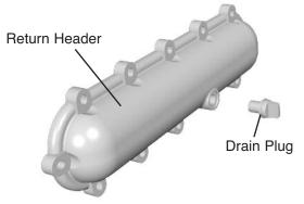
3. For ASME Heaters only: Disconnect compression fittings from the pressure switch and return header that connects to the 1/4" copper tube and allow the tube to drain.
