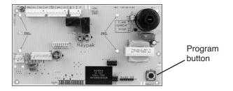
seconds. The heater will continue to operate normally while in the Service Menu. The first screen displayed is the Flame Strength indicator, which indicates the pilot flame current using a bar graph and numerical display. A signal of less than 4 indicates a weak flame signal and may require service. Refer to Section 5 – Troubleshooting for possible causes and corrections.
