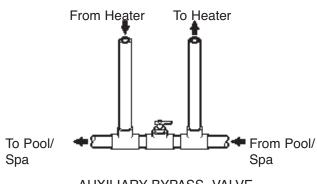
AUXILIARY BYPASS VALVE (DO NOT USE GATE VALVE)
