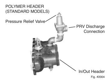
A 3/4" NPT connection is provided in the header for installation of a pressure relief valve. The valve shall be installed in a vertical position.
