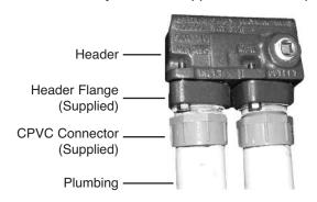
**WARNING:** NEVER install PVC directly into header flanges. Use the 2" CPVC adapter supplied loose with the heater.
