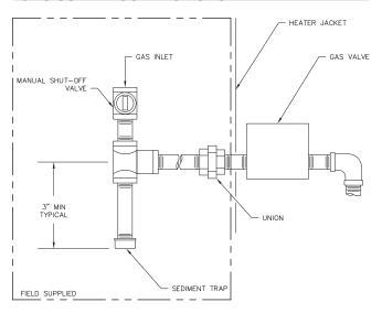
Gas piping must have a sediment trap ahead of the heater gas controls, and a manual shut-off valve located outside the heater jacket. All gas piping should be tested after installation in accordance with local codes.
