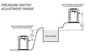
**NOTE:** If heater is installed outside of the limits shown, a higher pressure rated (11 psi) switch may be used. A flow switch, mounted and wired adjacent to the heater, may be used in place of the factory-mounted pressure switch. See Parts List (page 52) for 11 psi water pressure switch.
