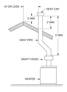
**NOTE:** With venting application of two or more heaters, contact the factory.
