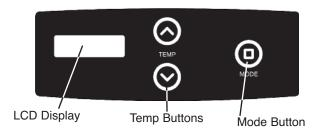
The pool heater touchpad, located on the upper front panel of the heater, allows the user to select either POOL or SPA operation, and to adjust the setpoint temperature. The LCD display window indicates the mode (OFF, SPA, POOL) and the actual water temperature. A manual power switch provided below the touchpad turns the control power ON or OFF.
