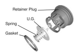
To test the operation of the Unitherm Governor, place in hot water (over 110°F) and watch for movement against spring. If there is no movement, replace unit.
