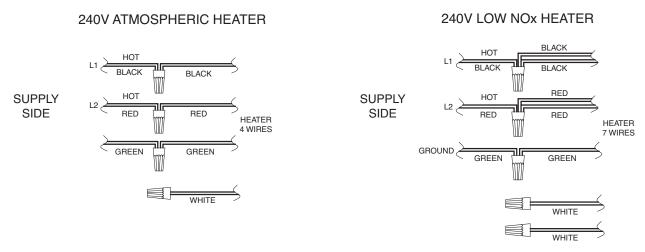
Heater must be electrically grounded and bonded in accordance with local codes, or, in the absence of local codes, with the latest edition of the National Electrical Code, ANSI/NFPA 70. (Canada - Canadian Electrical Code, CSA C22.1, Part 1 and Part 2.)
