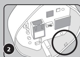
Using needle-nose pliers, remove the plastic break-away.
