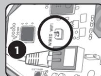
Remove the two screws from front cover. Remove the cover and gasket from the web-connect device. To clear Wi-Fi settings and enter Wi-Fi Setup mode, toggle the WIRED / Wi-Fi switch to WIRED then back to Wi-Fi.
