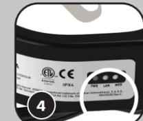
When connection to the home network is established, the yellow 'LAN' LED stops blinking and turns solid. When connection to the Internet is established, the green 'WEB' LED turns solid.
