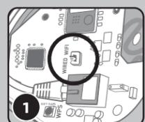
Remove two screws from front cover. Remove the cover and gasket from the web-connect device. To clear Wi-Fi settings and enter Wi-Fi Setup mode, toggle the WIRED / Wi-Fi switch to WIRED then back to Wi-Fi.
