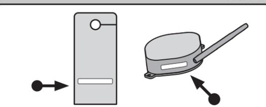
After creating an account, select the [+] in the top right corner (app) or "Add Location" tab (web). Enter the device serial number found on the door hanger or the side of the web-connect device.
