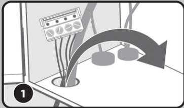
Turn off power to AquaLink. Remove the dead panel. Pass IQ30 web-connect device cable through the low voltage raceway.
