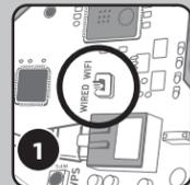
Remove two screws from front cover. Remove the cover and gasket from the web-connect device. To clear Wi-Fi settings and enter Wi-Fi Setup mode, toggle the WIRED / Wi-Fi switch to WIRED then back to Wi-Fi.
