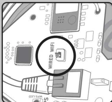
Remove the device lid by removing the two screws on the cover. To clear any previous Wi-Fi settings, toggle the Wired-Wi-Fi switch. Set the switch to the desired mode. Proceed to step 3.1 or 3.2 to reprogram the Wi-Fi settings.
