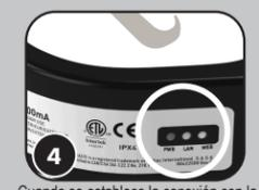
When connection to the home network is established, the yellow 'LAN' LED stops blinking and turns solid. When connection to the Internet is established, the green 'WEB' LED turns solid.
